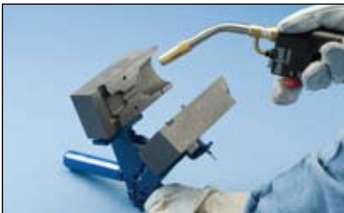
Fig. 10 Graphite absorbs moisture. Ignite the propane torch and dry out the inside of the mold thoroughly on both sides, heating the mold to approximately 250 degrees Fahrenheit (120 degrees Celsius).
