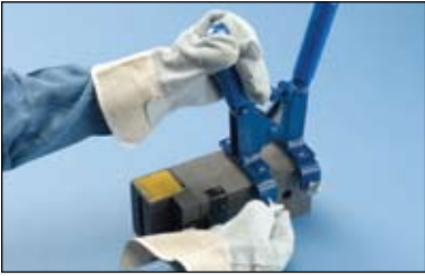
Fig. 7 Tighten the clamp thumbscrews onto the mold.
