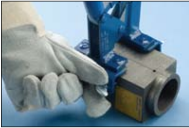
Fig. 7 Tighten the clamp thumbscrews onto the mold.
