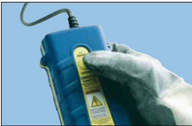
Fig. 13 Using the control unit, press the button and hold, while you observe the "ready" indicator light. A green light will blink for a few seconds and then will change to a constant light. At this time, the unit will send a charge to the ignition strip. The ignition strip will spark inside the metal cup, activating the CADWELD® PLUS exothermic reaction.
