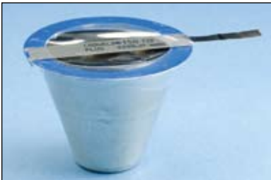
Fig. 15 Remove the proper CADWELD® PLUS welding material cup from the plastic container. Inspect the cup to ensure it is tightly sealed and the ignition strip is securely attached to the seal.
