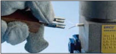
Fig. 25 Take the alligator clips and clip them onto the wire leads. Remove or protect fire hazards in close proximity to the connection. Advise nearby personnel of welding operations in the area.
