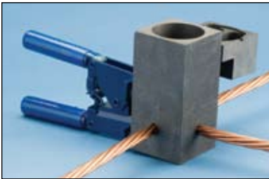
Fig. 14 Close the clamp tightly once the conductors are properly positioned.
